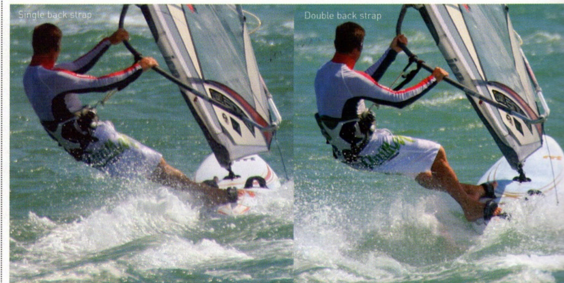
The single back strap helps keep your back leg straight even on a broad reach, whereas the double back strap will force your back leg to be bend
